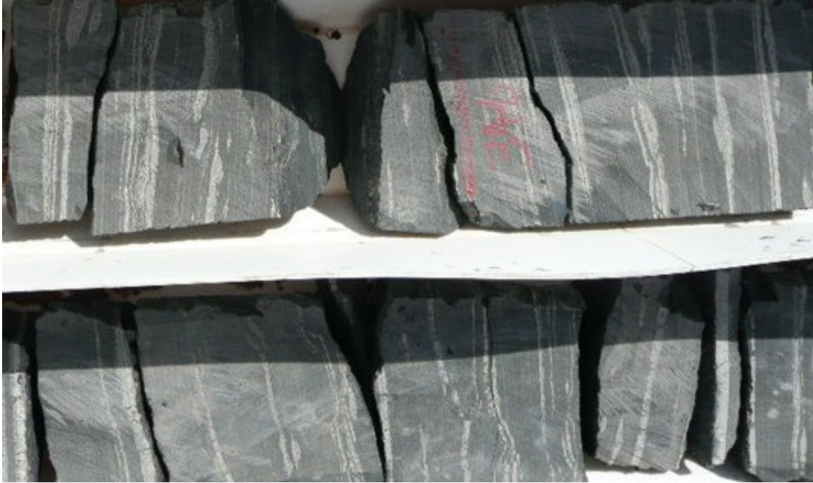
IHAD5 ~395-6 meters: Representative section of Tapley Hill Formation mineralized at 4.18% copper equivalent.
