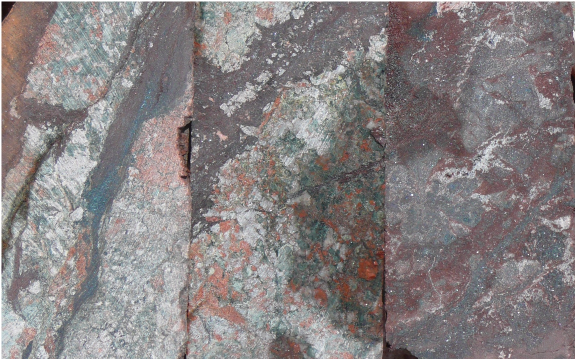
IHAD5 ~924-36 meters: Examples of bornite mineralized, chlorite- and hematite-altered brecciated granite.
