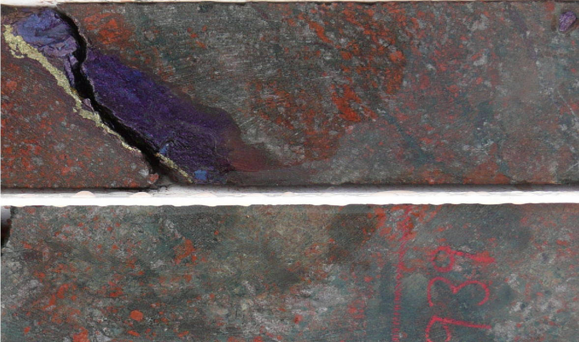
IHAD5 ~940 meters: Composite centimetric massive chalcopyrite-bornite vein and disseminated bornite in chloritized and brecciated granite host.
