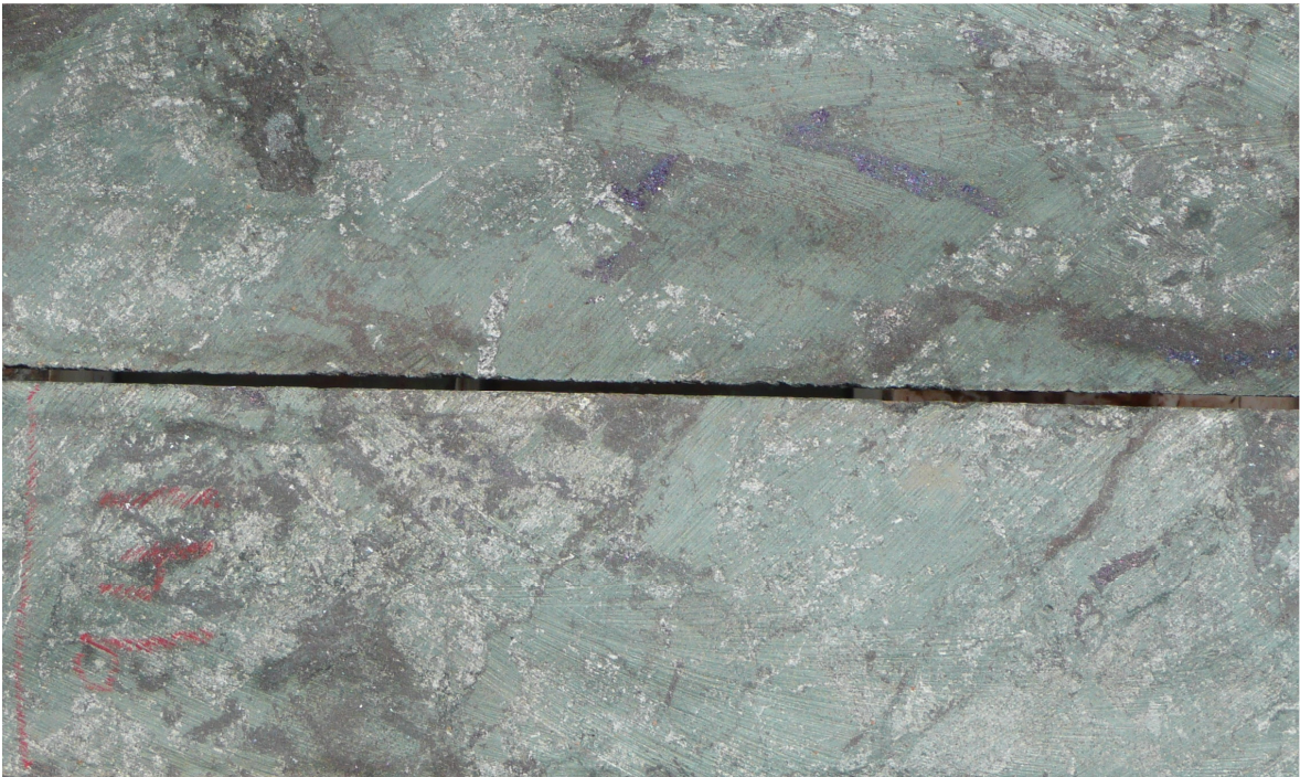
IHAD5 ~941 meters: Pervasively chloritized brecciated granite with hematite and bornite gash veins, aggregates and disseminations.
