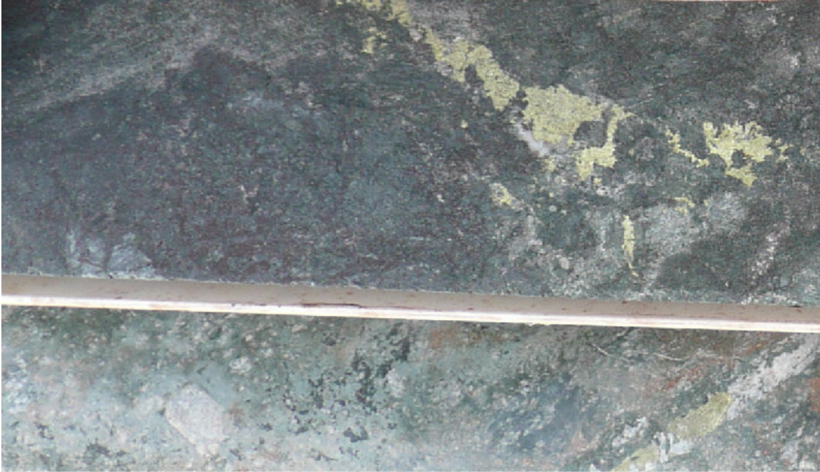
IHAD5 ~952 meters: Disseminations, aggregates and veins of chalcopyrite/pyrite in hematite- and pervasively chlorite-altered granite breccia host.
