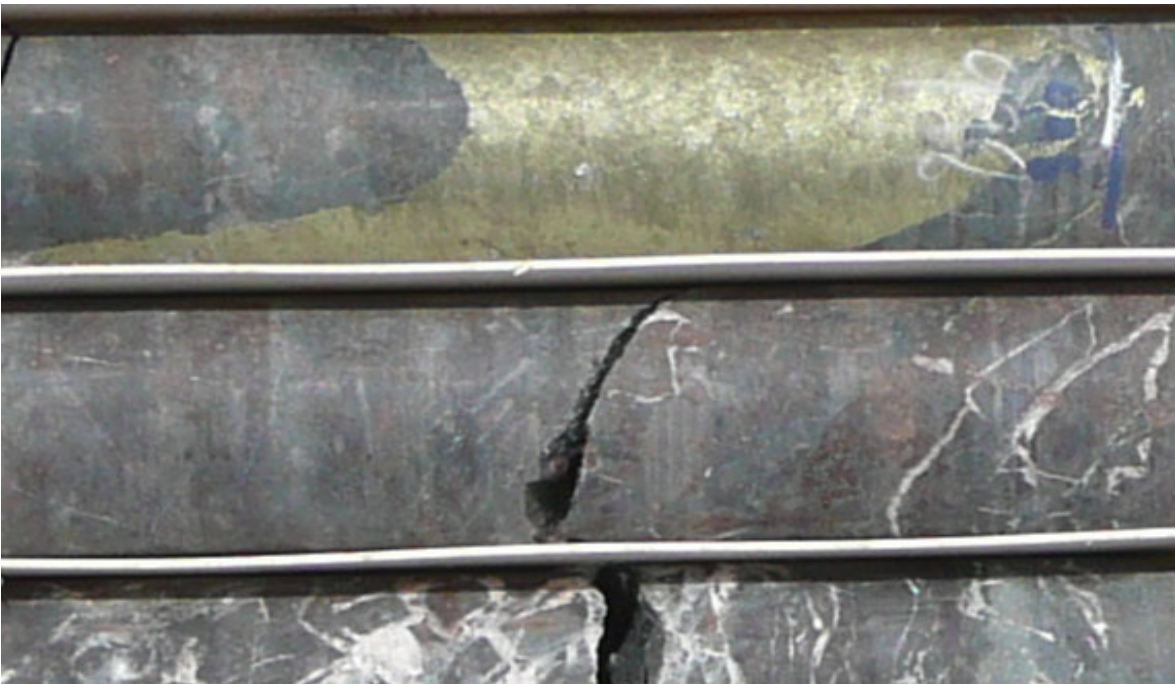
IHAD5 ~998 meters: Massive centrimetric chalcopyrite vein in strongly veined and brecciated, chlorite/hematite altered granite host.
